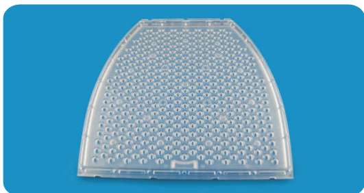
Item No.: HL-SD384W-K Angle: 75X140° Dim.: L325*W312*H10mm Material: PC
